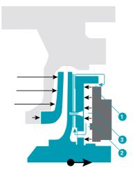
In the real functioning position, pressure in the chamber is regulated between high and low pressure. Resultant force is null and the mobile is stable and perfectly balanced between both.
